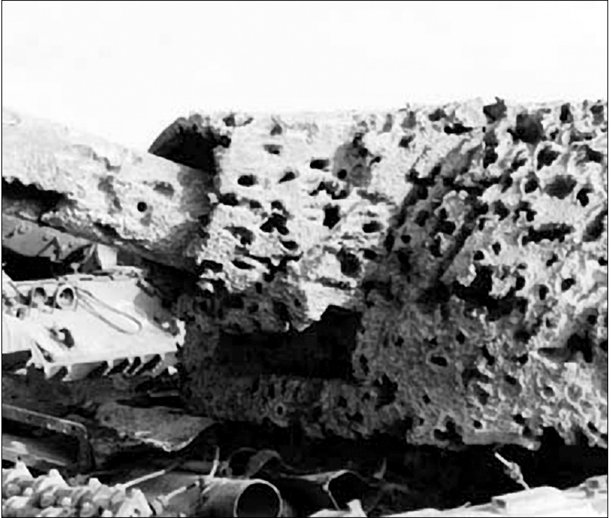
Image of a tank used for target practice. The holes burned through the steel are the result of depleted uranium munitions. Without exploding, the dU cuts through the metal while becoming small airborne particles. Take a deep breath...
